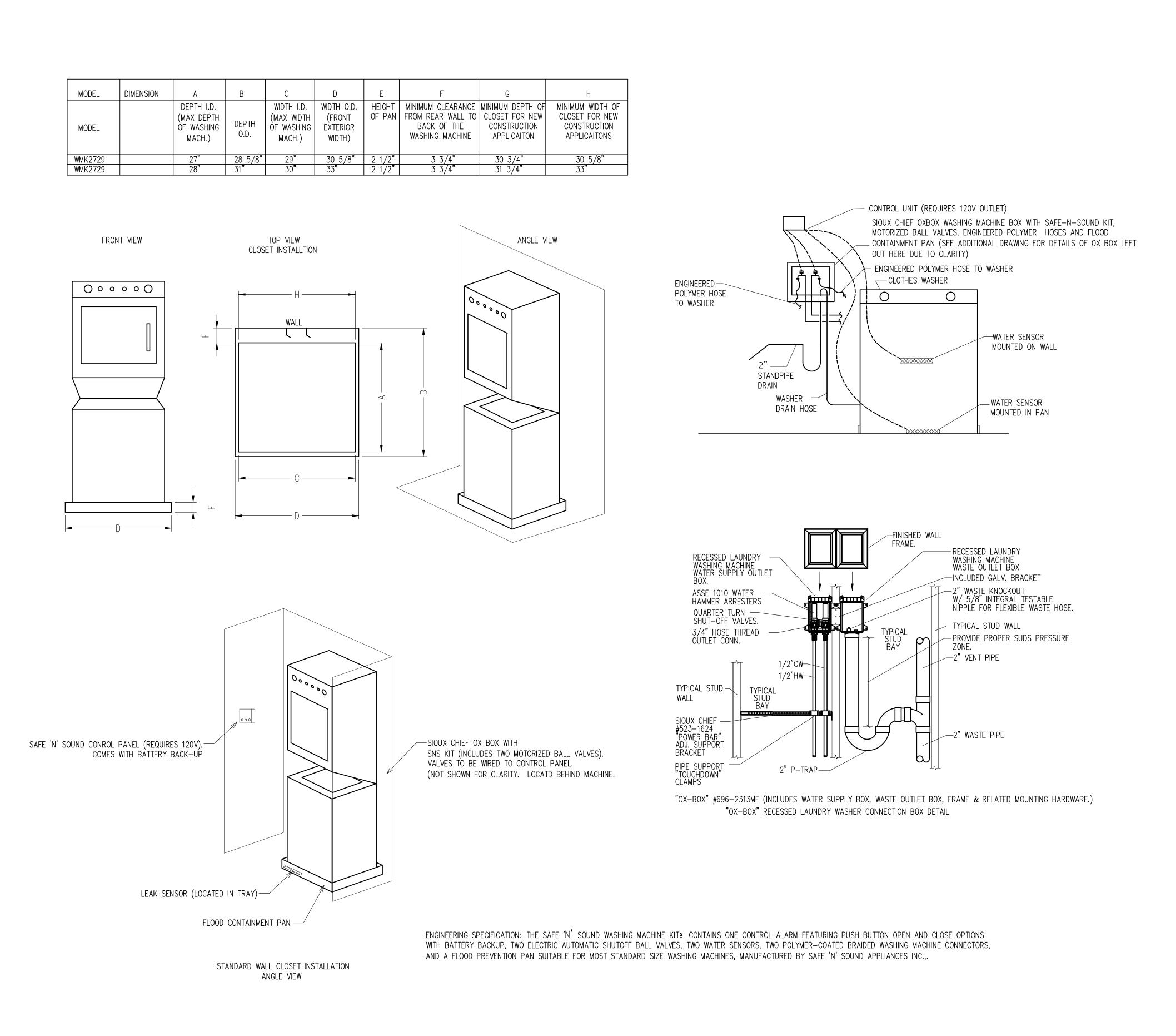
TYPICAL WASHING MACHINE CONNECTION DETAIL WITH FLOOD PREVENTION SYSTEM
